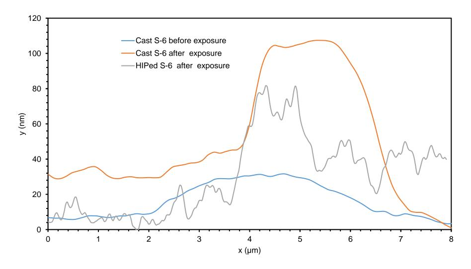
Figure 3. Line profiles from the AFM heights maps showing the height differences between the Co-rich matrix and the Cr-rich carbide in both the cast and HIPed S-6 for the conditions as marked as follows: cast S-6 before exposure (from Figure 2(b); cast S-6 after autoclave exposure (from Figure 7(c)); HIPed S-6 after autoclave exposure (from Figure 11(b).
