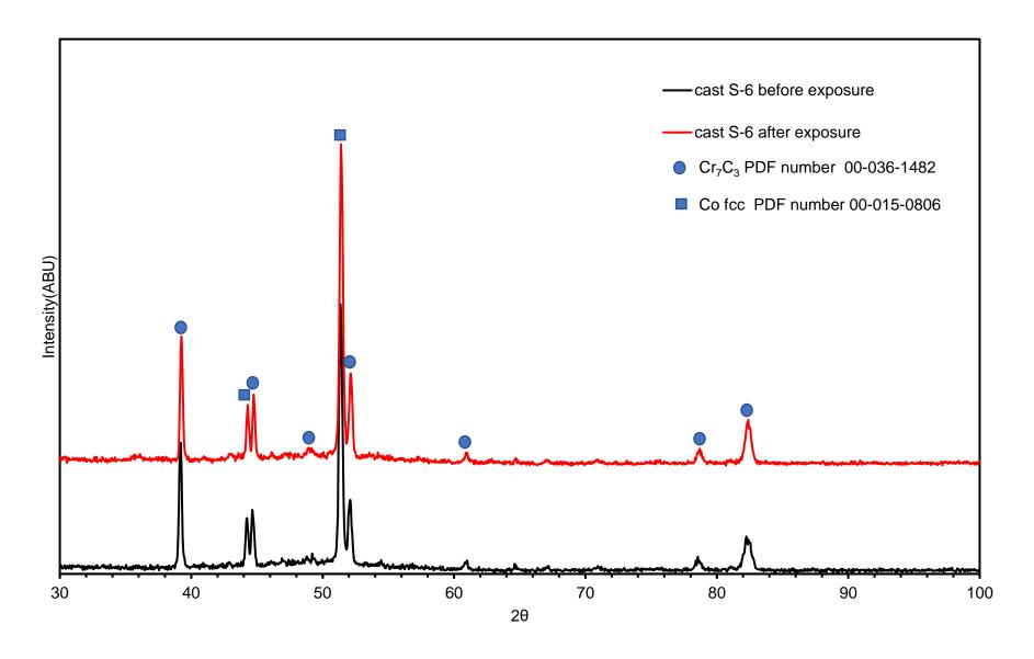
Figure 4. XRD patterns of cast S-6 both before and after autoclave exposure showing peaks associated with the two main phases.
