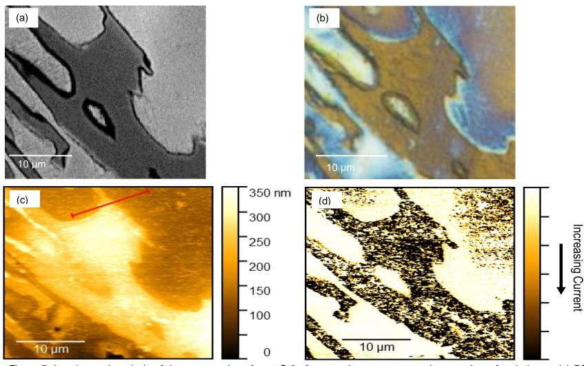
Figure 7. Imaging and analysis of the same region of cast S-6 after autoclave exposure, using a variety of techniques: (a) BSE-SEM image showing interfacial corrosion; (b) optical image showing interference colours associated with the corrosion products, with blue indicating a thicker corrosion product; (c) AFM tapping-mode height map with a line indicating the position of the height profile presented in Figure 3; (d) AFM contact-mode current map showing regions of higher current flow (dark).
