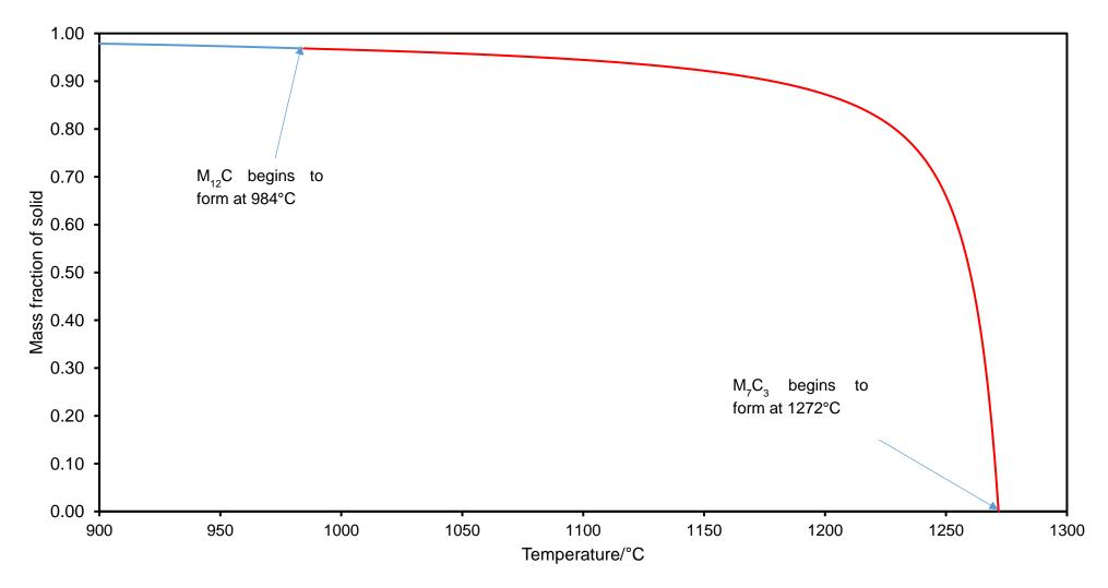
Figure 13(a). Predictions from Scheil–Gulliver solidification modelling of cast S-6: (a) mass fraction of solid as a function of temperature plot showing the temperatures at which particular phases began to be formed during the solidification sequence;
