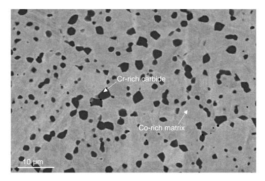
Figure 8. BSE micrograph of HIPed S-6 showing the two main phases.
