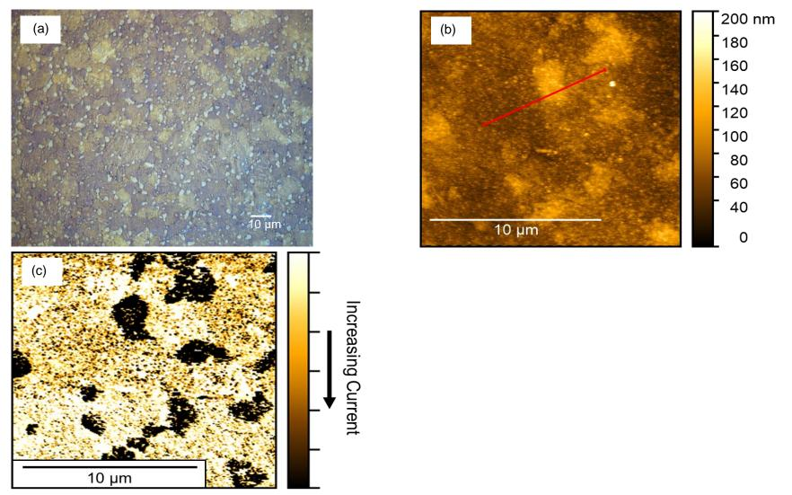
Figure 11. Imaging and analysis of HIPed S-6 after autoclave exposure: (a) optical image showing general region where AFM imaging was performed; (b) AFM tapping-mode height map with a line indicating the position of the height profile across Co-rich matrix with a Cr-rich carbide presented in Figure 3; (c) AFM contact-mode current map of the same area examined in (b).
