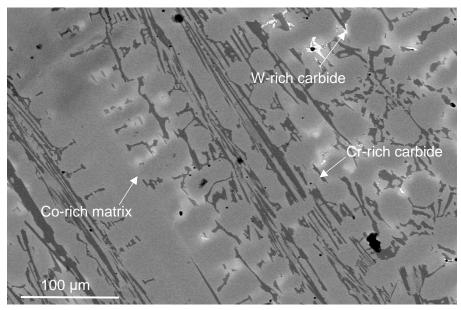
Figure 1. BSE Micrograph of cast S-6 showing the three main phases.
