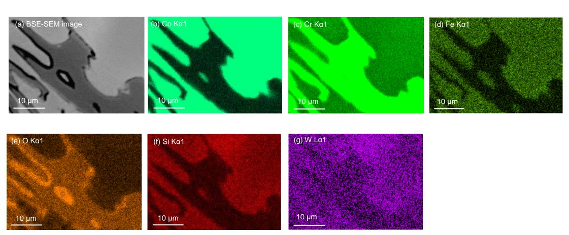
Figure 6. BSE-SEM image and EDX maps of cast S-6 after autoclave exposure examining the region highlighted in Figure 5(d): (a) BSE-SEM image; EDX maps of the following elements: (b) Co Kα1; (c) Cr Kα1; (d) Fe Kα1; (e) O Kα1; (f) Si Kα1; (g) W Lα1
