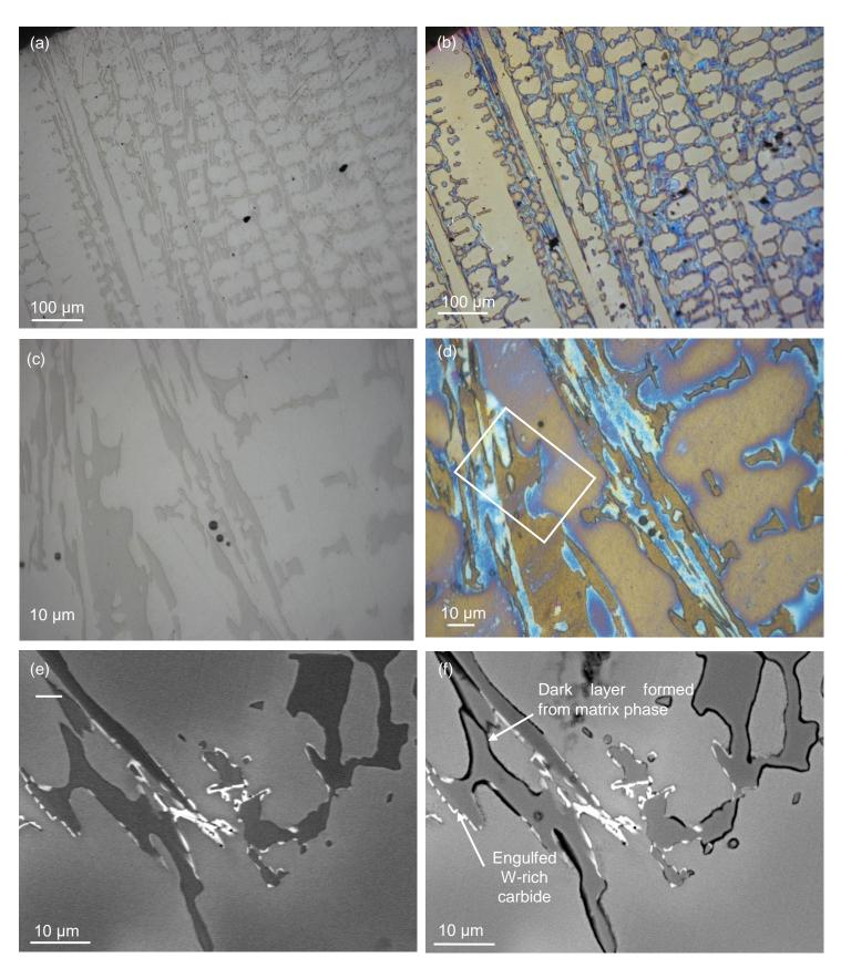
Figure 5. Image pairs of the same regions of cast S-6 before and after autoclave exposure; (a) and (b) low magnification OM images before and after exposure respectively; (c) and (d) high magnification OM images before and after exposure respectively; (e) and (f) BSE-SEM images before and after exposure respectively. The white box in (d) indicates the region where EDX mapping (presented in Figure 6) and AFM mapping (presented in Figure 7) was conducted
