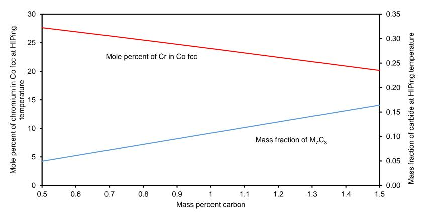
Figure 14. Predictions of variation in features (mass fraction of  $M_7C_3$  and the chromium content in the Co fcc phase) of the equilibrium microstructure at 1200°C in an alloy with the composition of HIPed S-6 but with the carbon level being allowed to vary (at the expense of the cobalt only).
