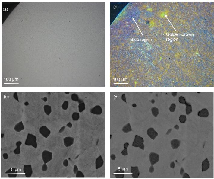
Figure 10. Image pairs of the same regions of HIPed S-6 before and after autoclave exposure; (a) and (b) low magnification OM images before and after exposure respectively; (c) and (d) BSE-SEM images before and after exposure respectively.
