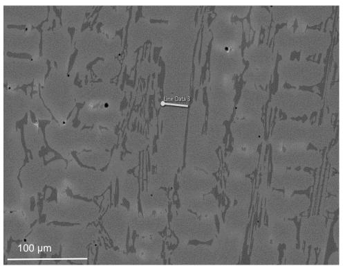
Figure 12(a). BSE image of cast S-6 of showing the line across a dendrite arm along which EDX analysis was made.
