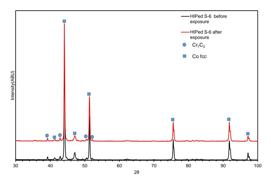
Figure 9. XRD patterns of HIPed S-6 both before and after autoclave exposure showing peaks associated with the two main phases.
