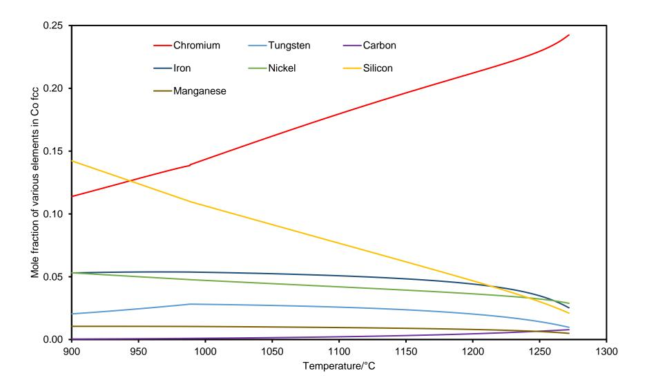
(b). composition of the Co fcc being formed at each temperature as solidification progresses (temperature being reduced
