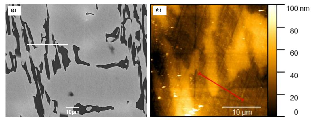
Figure 2. Imaging and analysis of cast S-6 before autoclave exposure: (a) BSE-SEM image with the region where AFM was conducted indicated by a white box; (b) AFM contact-mode height map with a line indicating the position of the height profile presented in Figure 3.
