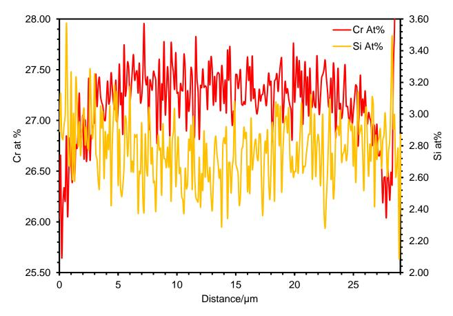
(b) compositions of chromium and silicon measured across the dendrite arm.
