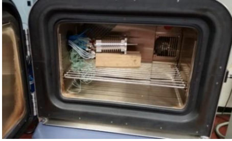
Fig. 12. Experimental setup for the thermal tests: PMSM equipped with thermocouples and placed inside the environmental chamber.
