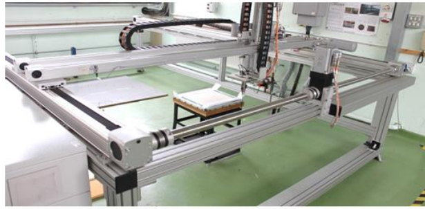
Figure 7: Off-axis tow placement machine
