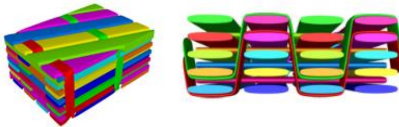
Figure 1: Meso-scale models of 3D reinforcements
