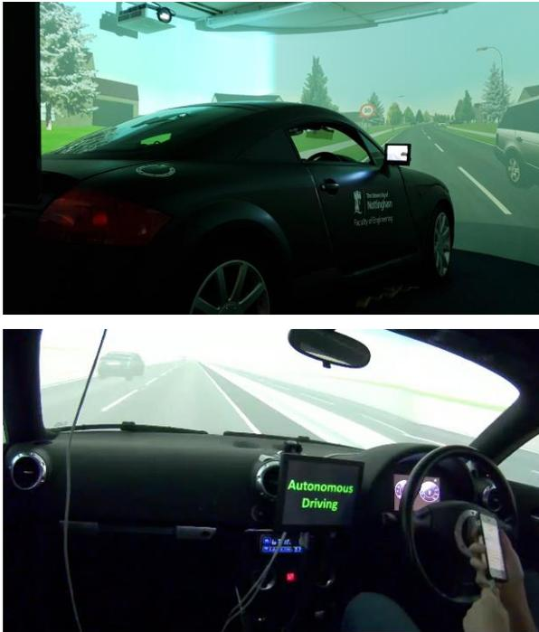
**Figure 1. University of Nottingham driving simulator, showing external (top) and internal (bottom) views**
