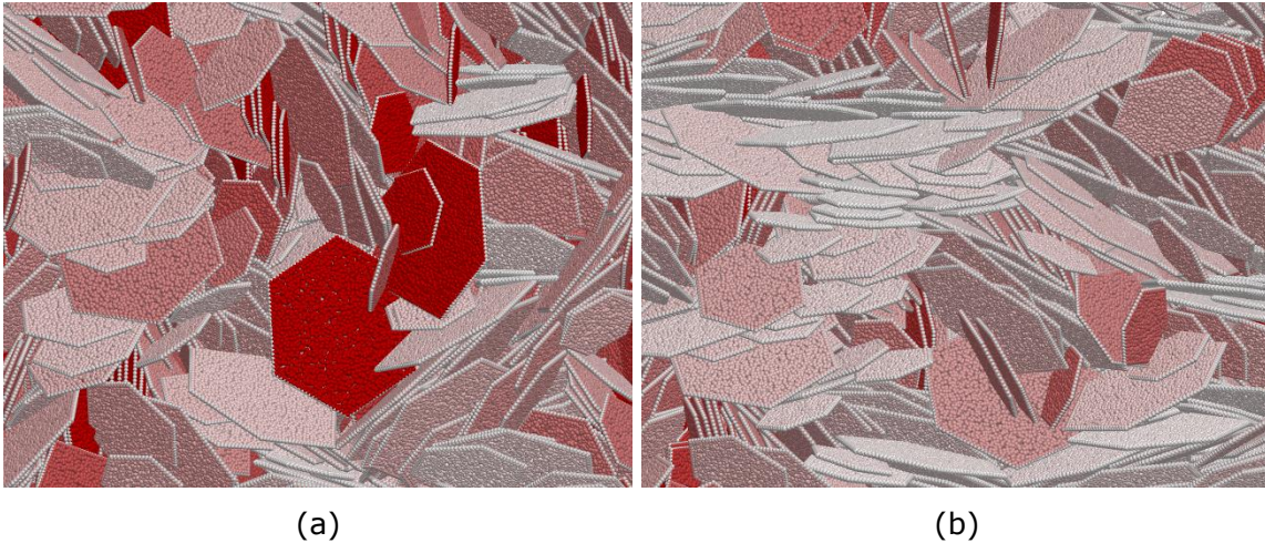
Figure 16. Cross sections showing internal platelet orientations before (a) and after (b) shearing at p=100 kPa. Darker red indicates more vertical orientation, white indicates horizontal orientation.
