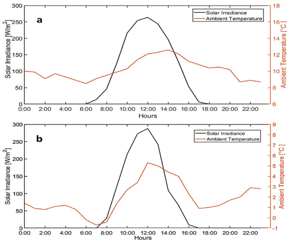
Fig. 6. EnergyPlus weather data for a) average day and b) cold day.
