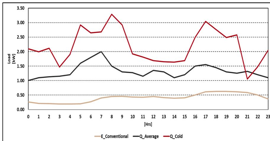
Fig. 2. The electricity and heat demand of a house.
