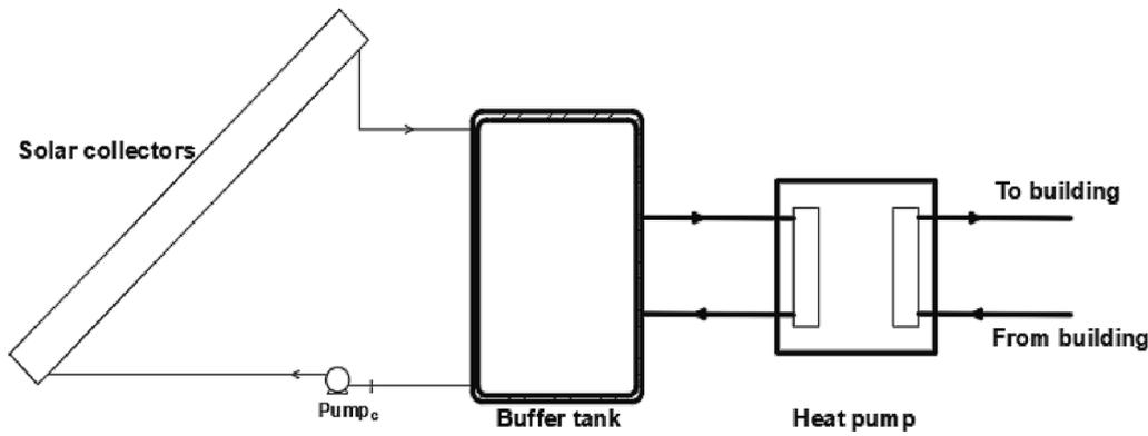
Fig. 3. Solar-assisted heat pump schematic.
