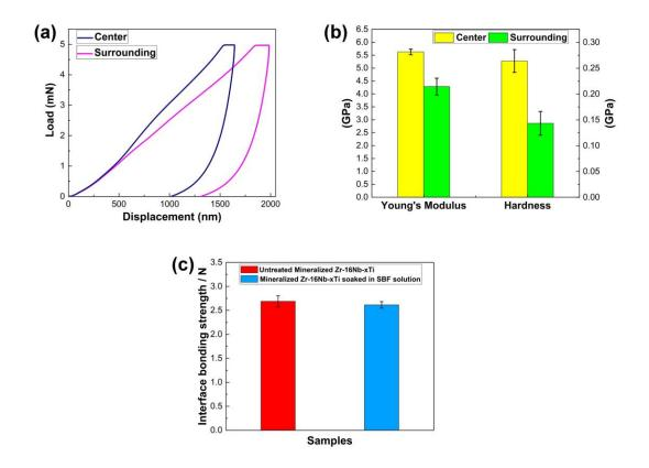
Figure 4. Nanoindentation analysis of mineralization structure with an ELR:HDI ratio of 1:12. (a) Displacement-load curves. (b) Young's modulus and hardness of the structure. (c) Bonding strength between mineralized coating and substrate under different conditions.
