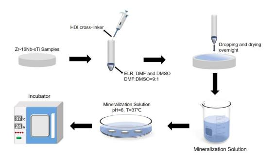
Figure 1. Schematic showing elastin-like recombinamer (ELR) protein membrane fabrication and mineralization process. DMSO, dimethyl sulfoxide; DMF, dimethyl formamide.
