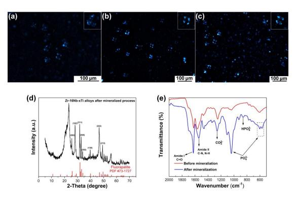
Figure 2. ELR spherulites and characterization of mineralized coatings. (a-c) Polarized light microscopy images confirm the presence of the ELR matrix within ELR membranes from Zr-16Nb-xTi (x=4,16 wt.%) alloy surfaces. (a) ELR:HDI=1:6. (b) ELR:HDI=1:12. (c) ELR: HDI=1:30. (d)
