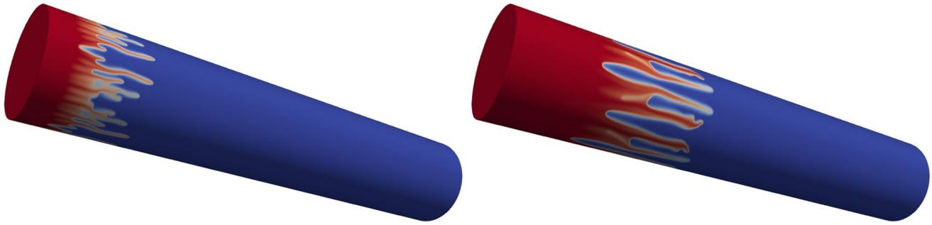
**Fig. 6** 3D viscous fingering at  $Pe = 10^3$  at dimensionless times 0.3 and 0.7. A high viscosity fluid (red) displaces a low viscosity fluid forming a fingering instability. As time passes the initially small
