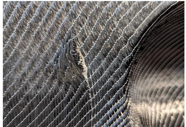
Fig. 22. In-plane fibre distortion, laddering, caused by anisotropic friction in the forming process.
