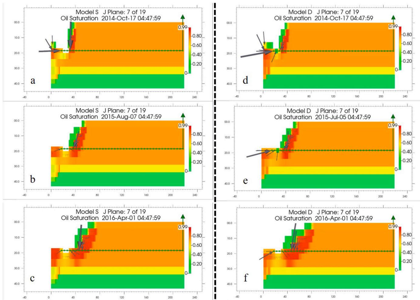
Fig. 21. Predicted oil saturation profile by model S and D during uninterrupted air injection period.
