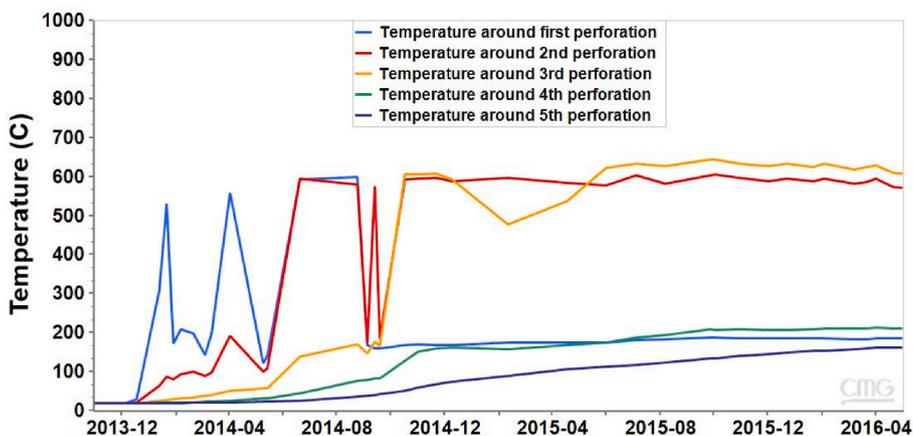
Fig. 8. Predicted variation of temperature around the toe section of HP in model S against time. Notes: \* Order of perforation is from the toe side of HP.
