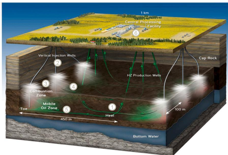
Fig. 2. Schematics of the Kerrobert THAI project (Petrobank Energy and Resources Ltd, 2012).
