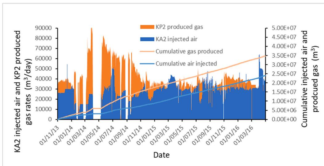
Fig. 4. The air injection profile, cumulative air injected, gas production profile, and cumulative gas produced for the K2 (form November 2013 to April 2016).
