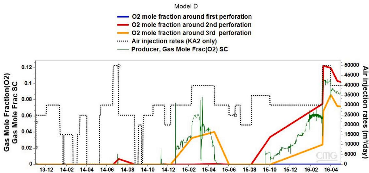
Fig. 15. Variation over time of injected air rates and predicted change in O2 concentration at toe section of the HP by Model D. Notes: \* Order of perforation is from the toe side of the HP.
