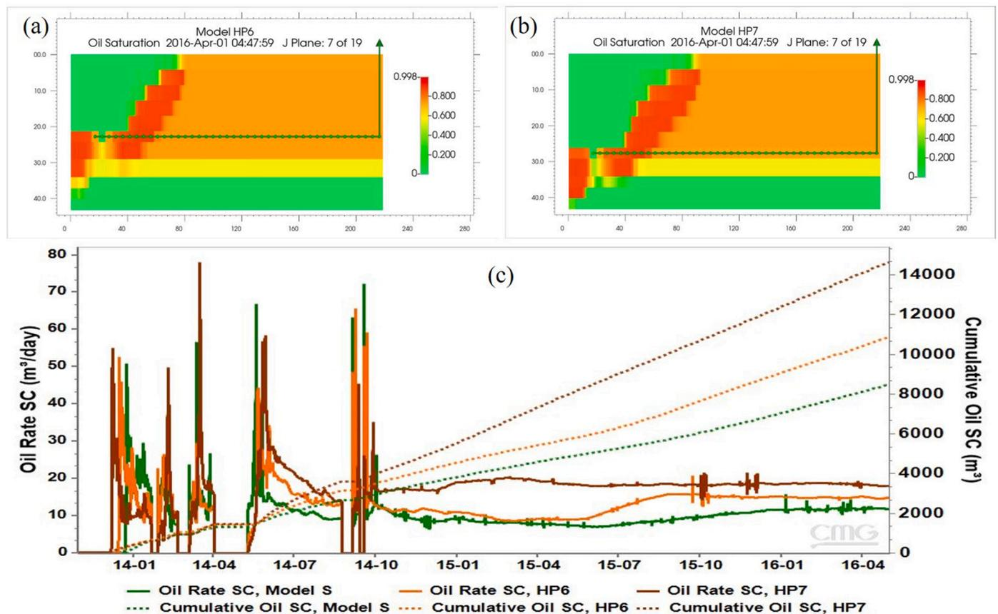
Fig. 22. Predicted oil saturation profile (a and b) and oil production profile by model S with varied HP location (c).
