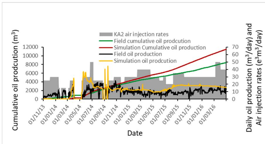
Fig. 9. Model D simulated oil production profile compared with corresponding field data for K2.
