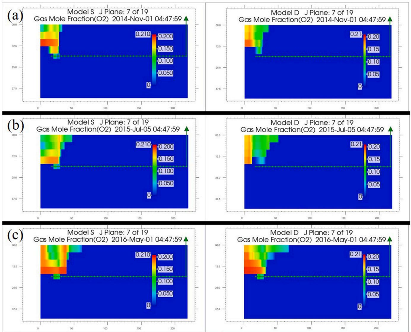
Fig. 13. Change in predicted oxygen profile for Model S (left) and Model D (right) at vertical midplane from November 2014 to May 2016 (uninterrupted air injection period).
