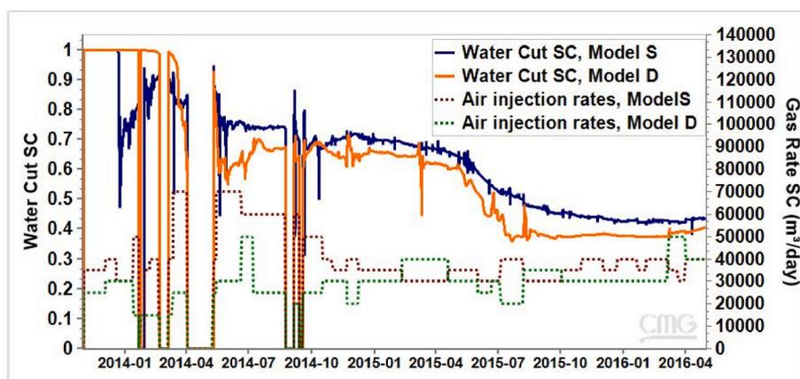
Fig. 10. Simulated water cut against air injection rates for Model S and Model D.
