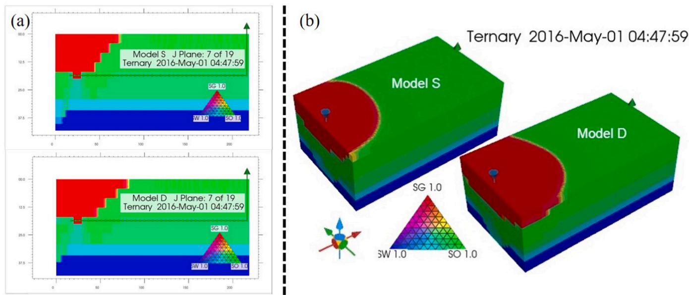
Fig. 12. Simulated ternary profile for model S and D in vertical midplane view (a) and in 3D (b) in May 2016. Notes: \* SO, SW, and SG represent oil saturation, water saturation, and gas saturation, respectively.
