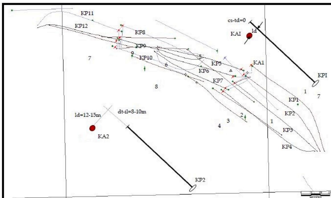
Fig. 1. The location of THAI well pairs (K1–K12, where KA is vertical injector and KP is horizontal producer). Old horizontal wells are marked from 1 to 9 (Turta et al., 2018).
