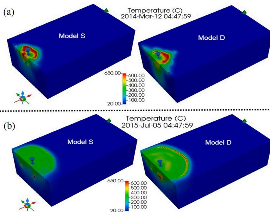
Fig. 17. 3D simulated temperature profile by Model S and Model D in (a) March 2014 and (b) July 2015.
