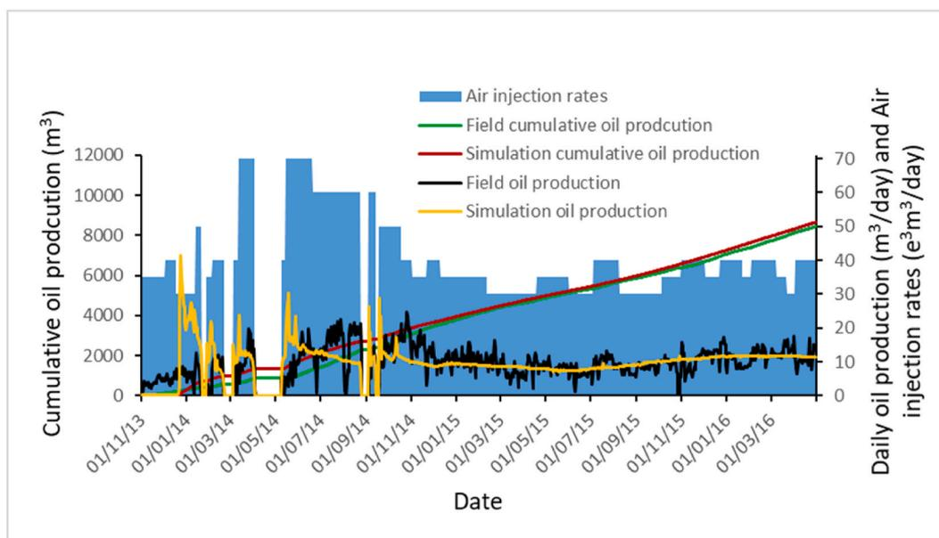
Fig. 6. Comparison of simulation results for Model S with field data for the K2 pilot.
