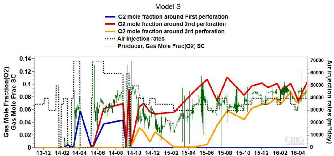
Fig. 14. Variation over time of injected air rates and predicted change in O2 concentration at toe section of the HP by Model S. Notes: \* Order of perforation is from the toe side of the HP.
