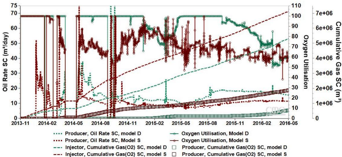
Fig. 16. Cumulative oxygen injected, cumulative oxygen produced, predicted oxygen utilisation, and oil production profile by Model S and Model D. Notes: \* The illustrated parameters are distinguished with different line styles.
