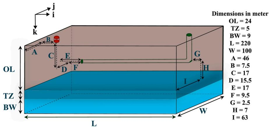
Fig. 5. Reservoir model dimensions and VI and HP configuration in quasi-staggered line drive (SQLD) fashion. Notes: \*The oil layer (pay zone), transition zone, and bottom water zone are shown in grey, dark blue, and light blue, respectively. (For interpretation of the references to colour in this figure legend, the reader is referred to the Web version of this article.)
