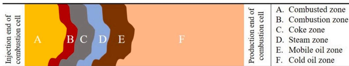
Fig. 11. Areal schematic of zones developed in the THAI process.
