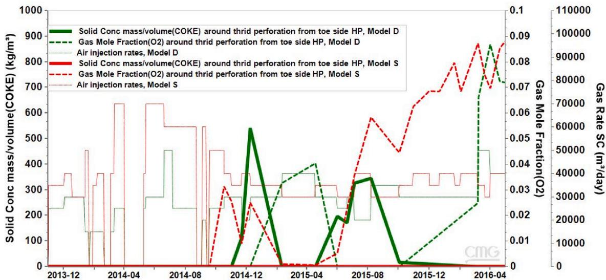
Fig. 19. Predicted coke concentration and oxygen profile around the third perforation from the toe side of HP in Model S and Model D. Notes: \*SC stands for standard condition.
