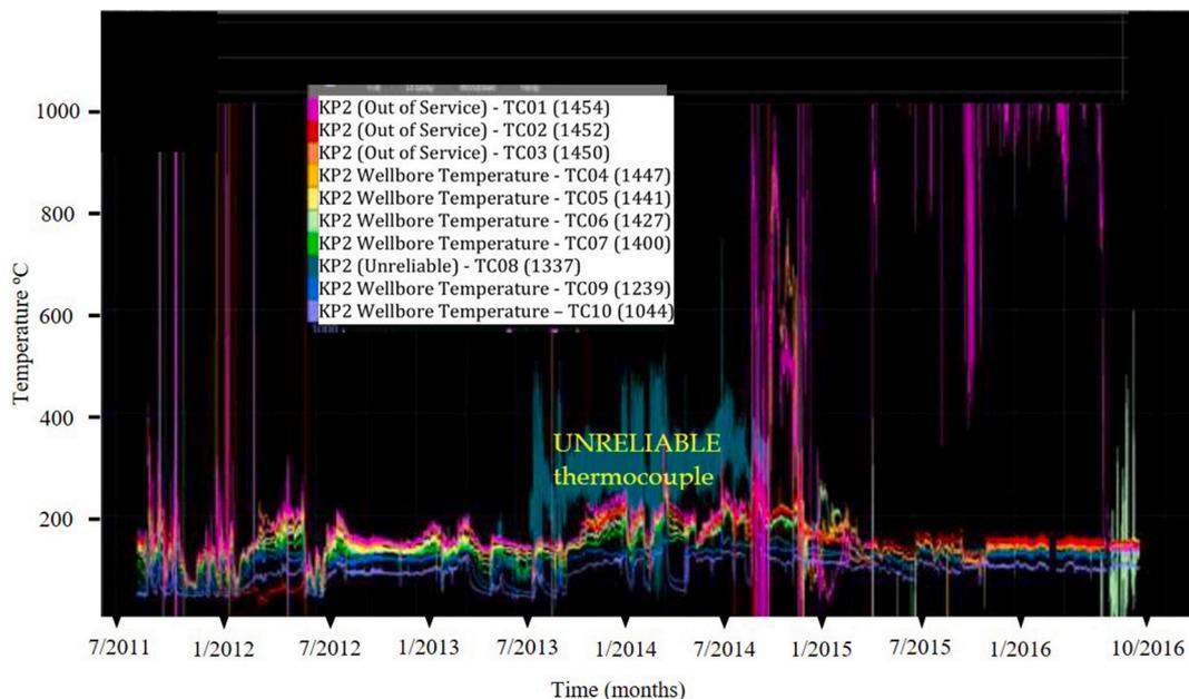
Fig. 7. Actual variation of temperature along KP2 versus time. Notes: \* TC01 is located at the toe of HP.
