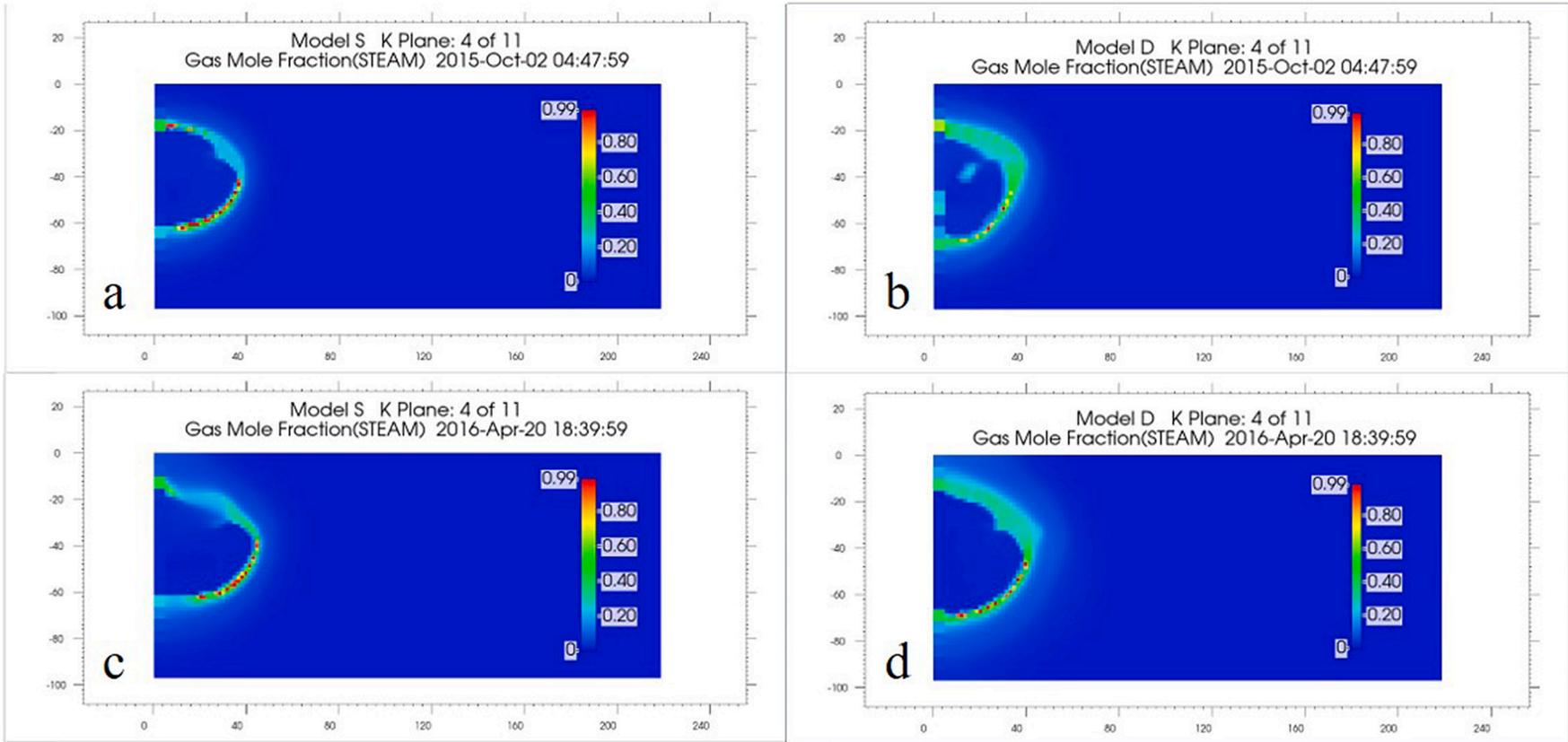
Fig. 20. Predicted steam profile by model S and D during THAI process.
