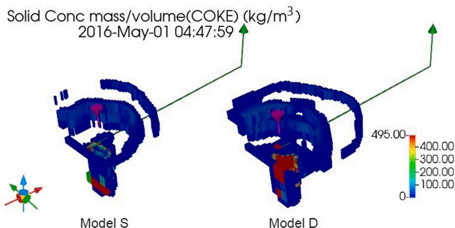
Fig. 18. Simulated 3D structure of the coke zone in Model S and Model D in May 2016.
