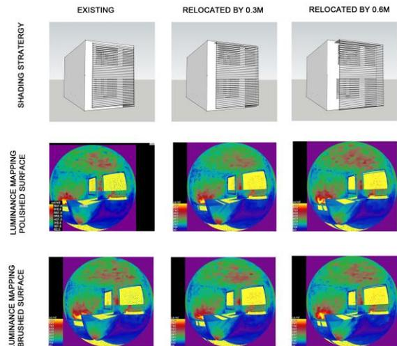
Figure 8: Shading device and Luminance mapping
