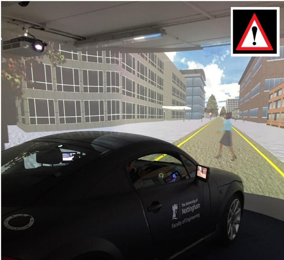
**Figure 1: Driving simulator showing urban high-street scenario and pedestrian crossing road ahead, with visual alert icon that was presented on the HUD (inset).**
