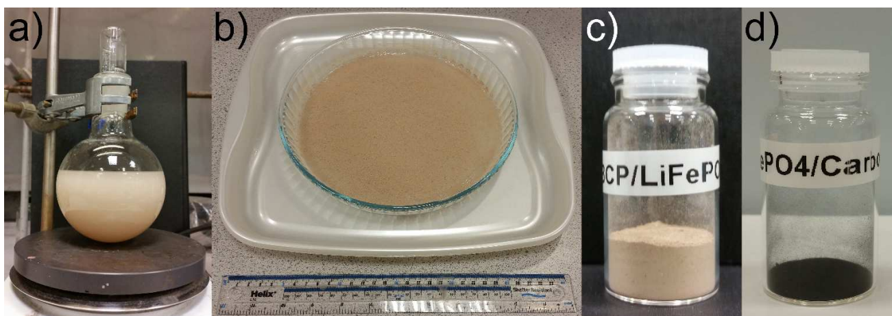
Figure S2. Photos taken during the scaled up (20 fold) synthesis of the BCP templating process with LiFePO 4 . 1 gram of BCP was used in this reaction. a) BCP slurry in ethanol after mixing with the combined sol-gel precursor solution. b) The LiFePO 4 infused BCP microparticles obtained as a dry powder on the surface of the glass drying dish. The ruler in the image is 30 cm long. c) Vial containing the BCP/metal oxide hybrid microparticle powder collected from the dish after drying. d) Vial with the pure LiFePO 4 /carbon microparticles collected after calcination in a tube furnace at 500 °C for 2 hours.
