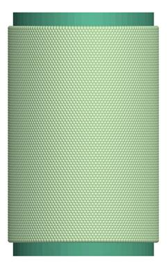
Fig. 4. Image of the triaxial sample with randomly colourised clumps to model particles (left) and bonded spheres to model the lateral flexible membrane (right).
