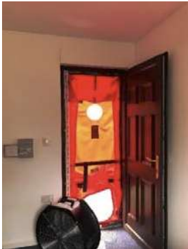
Figure 4 Setup of blower door model 4 (BD-4)
