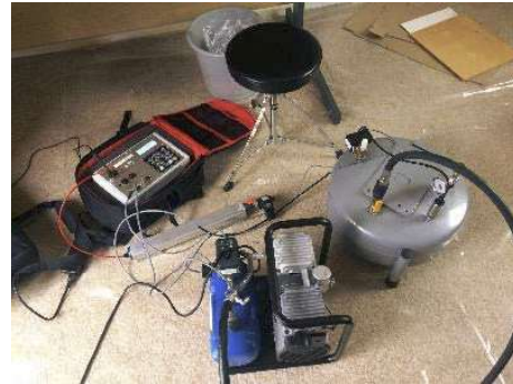
Figure 5 Setup of PULSE unit (PULSE-20)
