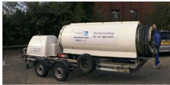
Figure 4 a petrol driven multi-gear portable trailer fan
