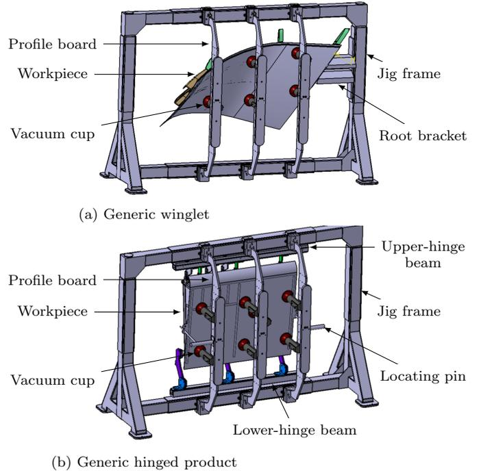
Fig. 1. Reconfigured jig for two different products
