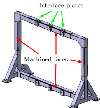
Fig. 4. Profile board connection upper interface to the jig frame
