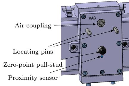
Fig. 5. Interface plate upper design
