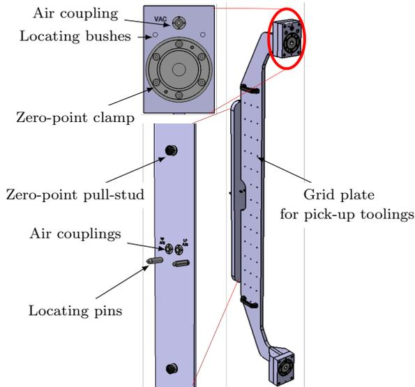
Fig. 7. The profile board with connection features to the jig frame and the end effector
