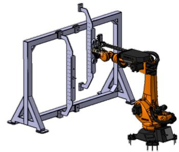
Fig. 2. PnP process: Robot load and unload profile boards onto the jig frame
