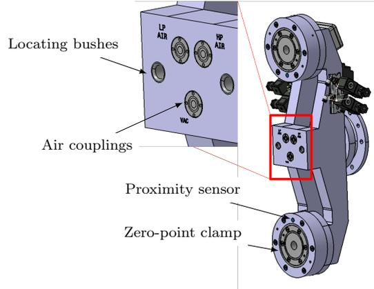
Fig. 8. PnP end effector with detailed service interface
