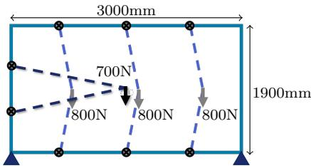
Fig. 3. Jig frame simplified loading condition
