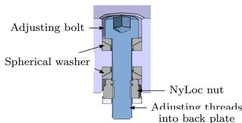
Fig. 10. NyLoc nut and spherical washer cross-section
