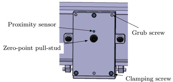
Fig. 6. Interface plate lower design
