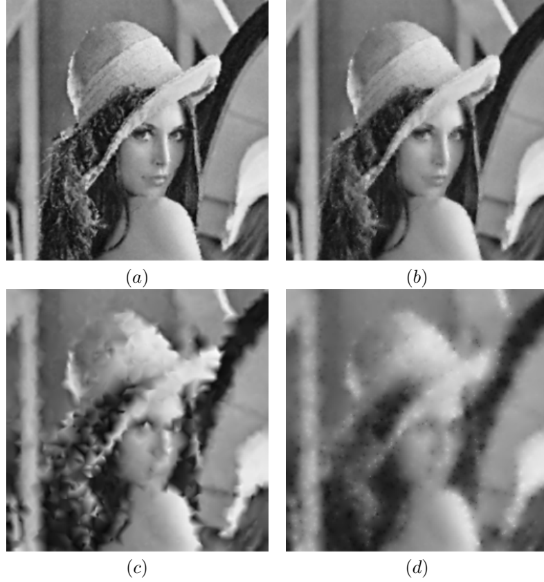
FIGURE 30. Example 7.2.5. Restoration of 90% corrupted image (PSNR = 5.901 dB) by: (a) Restored image A_\lambda^M(f_K) , with K the set of the pixels not corrupted by the salt & pepper noise when the corrupted image is enlarged symmetrically by two pixels on each side, \lambda = 15 and M = 1E13 . PSNR = 27.506 dB. (b) Restored Image by the two-stage TV-based method described in [12, 14] with the same set K as in (a). PSNR = 26.564 dB. Restoration of 99% corrupted image (PSNR = 5.492 dB) by: (c) Restored image A_\lambda^M(f_K) , with K the set of the pixels not corrupted by the salt & pepper noise when the corrupted image is enlarged symmetrically by ten pixels on each side, \lambda = 15 and M = 1E13 . PSNR = 21.972 dB. (d) Restored Image by the two-stage TV-based method described in [12, 14] with the same set K as in (c). PSNR = 20.492 dB.
