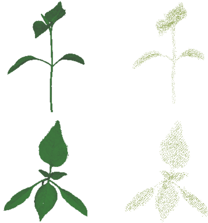
Figure 8 Experiment five conducted on a chilli plant ( Capsicum sp. ). The first column is the X-Ray data, obtained using a CT scanner, the top row presents a side view and the bottom row a top down view. The second column is a point set obtained using the AVC proposed here.
