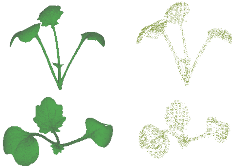
Figure 7 Experiment four conducted on Brassica napus . The first column is the X-Ray data, obtained using a CT scanner, the top row presents a side view and the bottom row a top down view. The second column is a point set obtained using the AVC proposed here.
