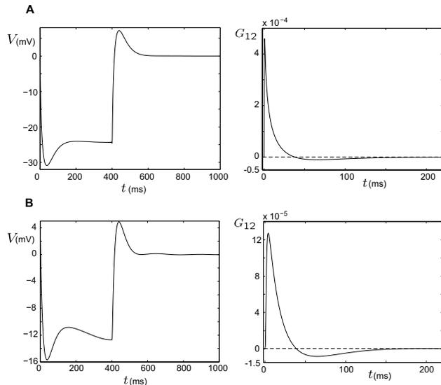
Figure 4: Examples of voltage profiles and Green's functions on branch 1 at the location  $X = 250 \mu\text{m}$  in response to the current with amplitude  $-0.3 \text{ nA}$  and duration of  $400 \text{ ms}$  injected on branch 2. A: Stimulus location is  $Y = 0 \mu\text{m}$ . B: Stimulus location is  $Y = 500 \mu\text{m}$ . Other parameters as in Figure 3.
