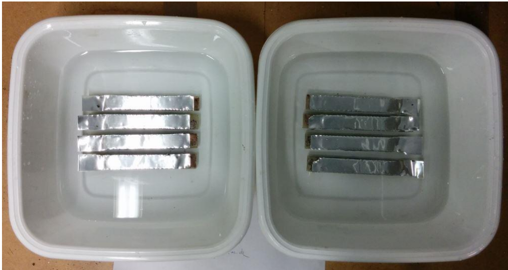
Figure 3. Moisture conditioning of adhesion specimens
