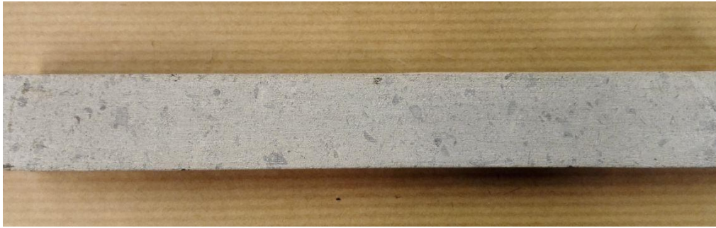
Figure 2. Aggregate substrate prepared from large boulders
