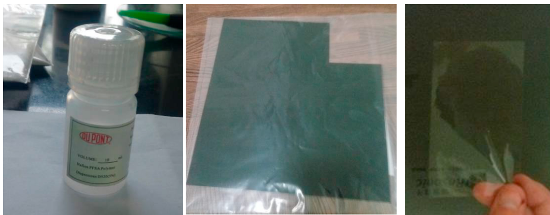
Fig. 2. Nafion 117 solution, GDL and Nafion 115 membrane
