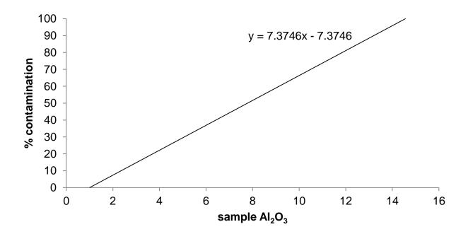
**Figure SI-1** Regression line showing equation used to derive Eq. 2: a mixing line between the point when  $Al_2O_3$  is 14.56% indicating 100% contamination and when  $Al_2O_3$  is 1% indicating 0% contamination (i.e. 100% diatom).
