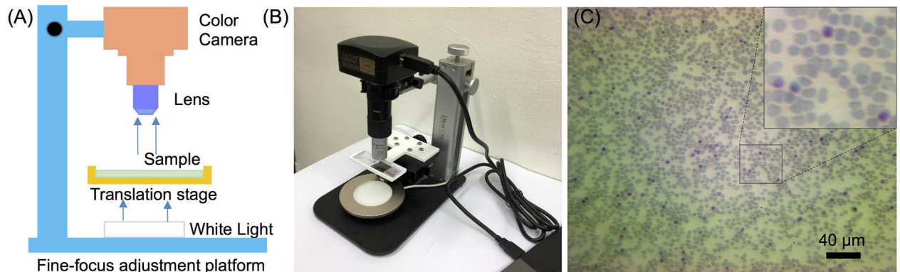
Fig 1. The developed image-based cytometer. (A) Schematic experimental setup of the cytometer. (B) Photograph of the image-based cytometer. (C) An image of the blood smear taken by the cytometer.
