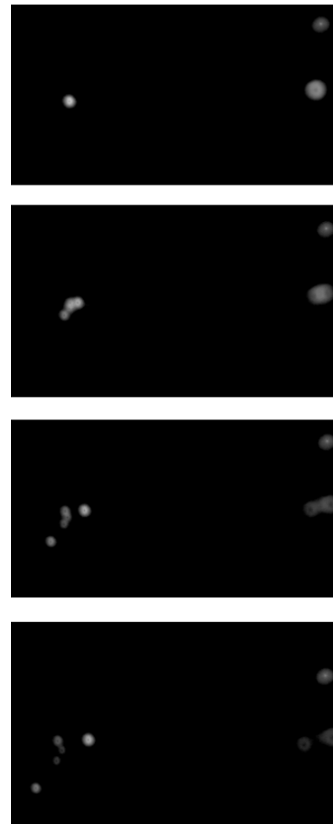
Figure 5 – Sections of four successive frames showing exploding particles during 500 W, 2 bar drilling.
