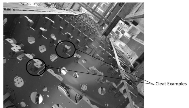
Fig. 2 Showing Butterfly brackets bolted onto wing ribs
