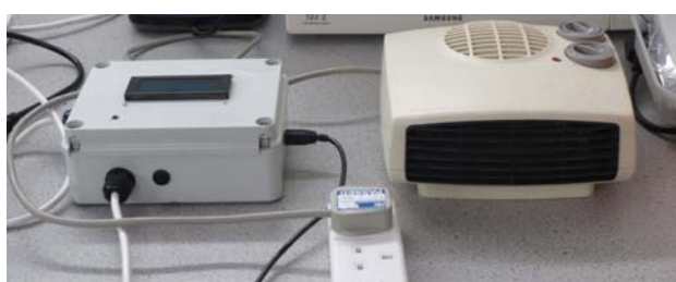
Figure 5. The receiver circuit under test with a small fan heater as load.
