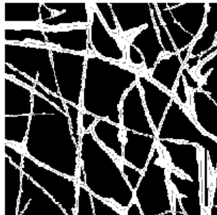
f. Centerline determination from SEM image
