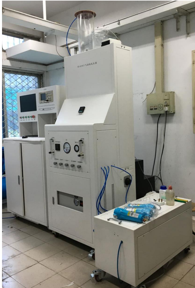
3 Fig. 3. Tester for classification filtration efficiency and pressure drop of filters (SX-L1060).
