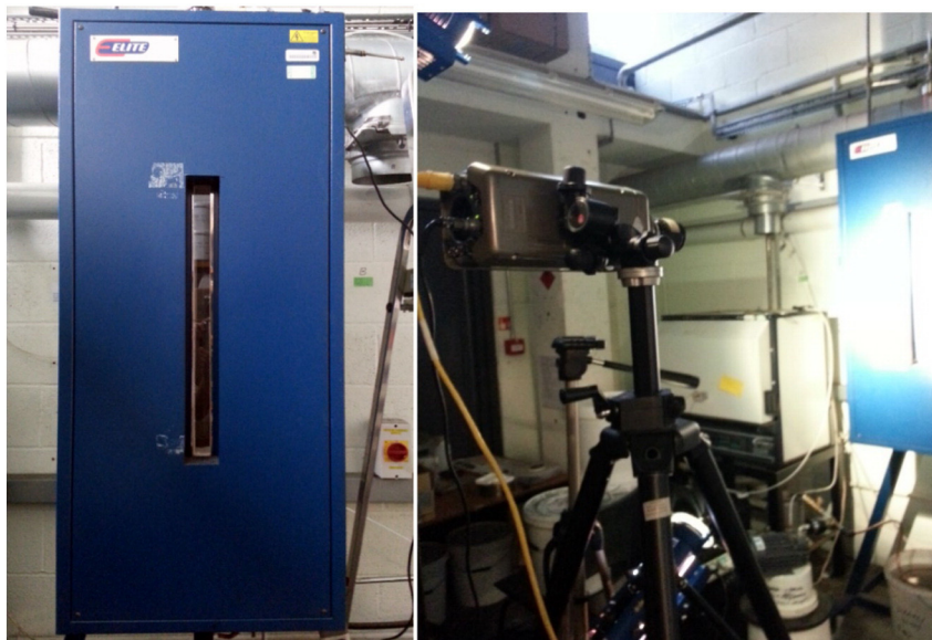
Fig. 1. Visual Drop Tube Furnace with a long viewing window (left) and video capture set-up showing Phantom V12.1 high speed camera with 105 mm Nikon lens (right).
