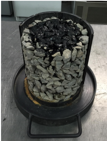
Fig. 4. Visual appearance of the stabilized ballast after emulsion setting.
