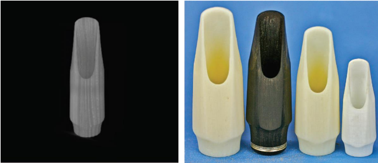
Figure 7. Left: XCT data of a saxophone mouthpiece, right: AM reproduced saxophone mouthpieces with original wooden mouthpiece (second from left). All the AM mouthpieces were produced by scaling of the original scan data and the rightmost mouthpiece was stated to be sufficiently dense as to operate successfully. Images reproduced from [66].
