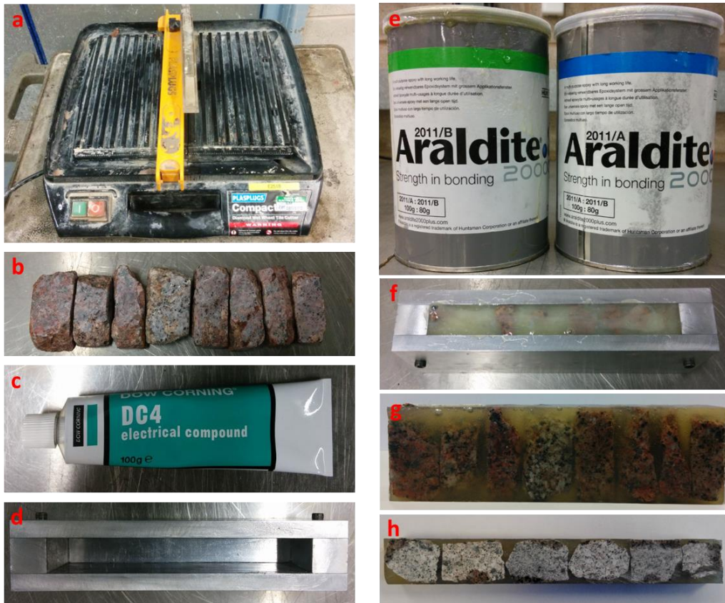
1 Figure 3. Procedures for aggregate substrate preparation: (a) trim saw, (b) aggregates after 2 trimming, (c) release compound, (d) assembled mould, (e) epoxy resin, (f) combine trimmed 3 aggregates in the mould and fill the gaps with epoxy resin, (g) cured composite aggregate, (h) 4 composite substrate used for peel test. 5 6 7 8
