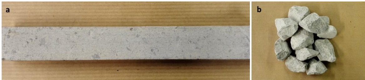
Figure 1. Aggregate substrate and coarse aggregates: (a) substrate must be prepared from large boulders, while (b) coarse aggregates are readily available in most labs.
