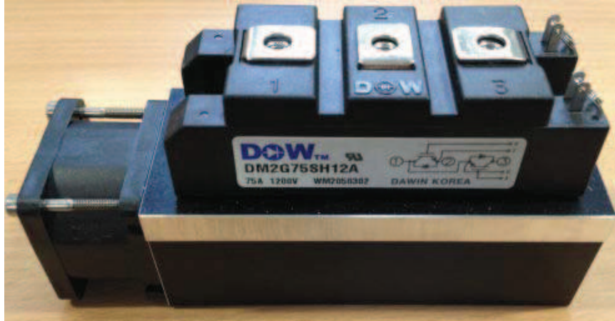
Figure 7: Tested IGBT module on heat-sink
