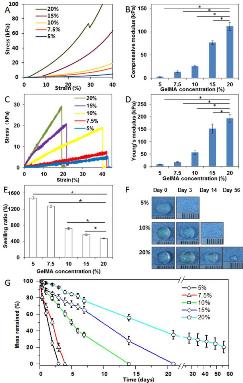
**Figure 1.** Compressive stress-strain characterization (A), compressive modulus (B), tensile stress-strain curves (C), tensile modulus (D), swelling ratio (E), representative photographs of morphology changes during *in vitro* degradation (F) and mass retention during degradation (G) of GelMA hydrogels of varying concentrations. Note that about 25% of 20% GelMA remained after 56 days of degradation study. \* indicates  $p < 0.05$ .
