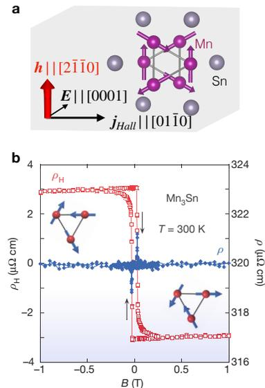
FIG. 1. **Experimental discovery of the Hall-effect in the compensated non-collinear magnet  $Mn_3Sn$ .** **a**, Crystal and magnetic structure of  $Mn_3Sn$ , and the Hall effect geometry. **b**, Magnetic field dependence of the Hall resistivity (left axis) and the longitudinal resistivity (right axis). Strong magnetic fields align magnetic moment in time-reversed states (insets). Panel b is adapted from Ref. 22.
