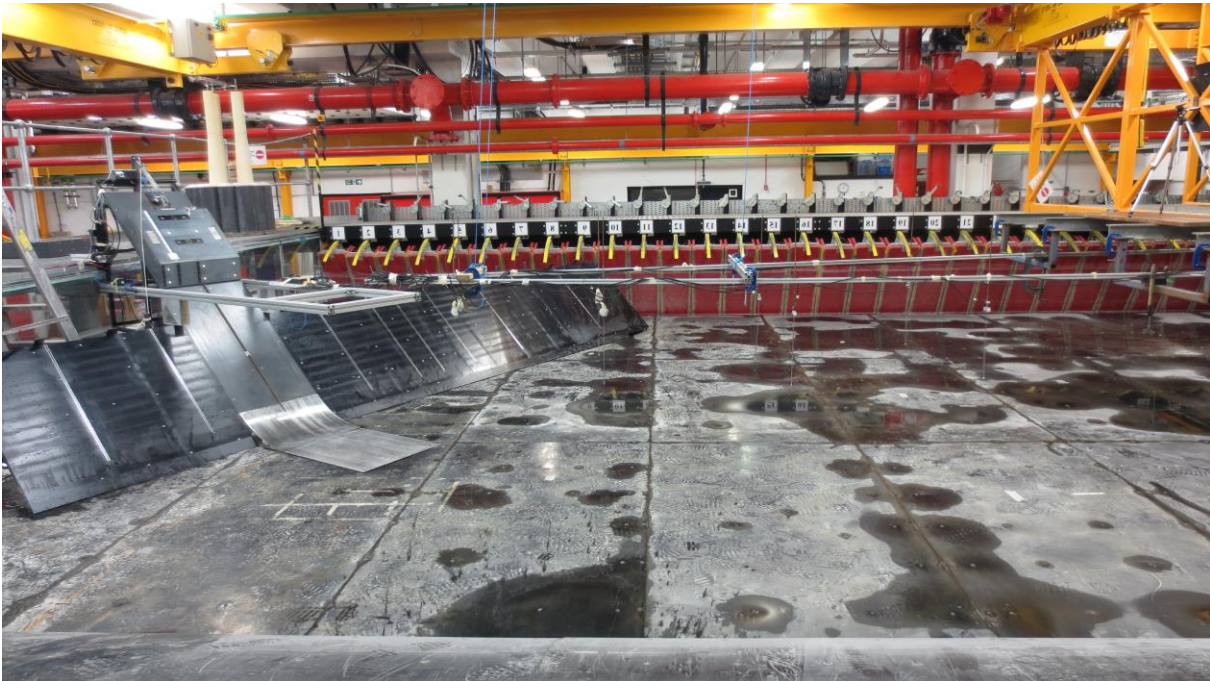
Fig. 1. Wave basin set-up in position 2 showing on the left: medium slide on ramp, circular transition and steel plate on ramp toe and side-walls with run-up gauges; centre: first wave probes at r/h = 3.0, 5.0, 7.5 and 10.0 for \gamma = 30^\circ and 45^\circ and h = 0.480 m; right: bridge supporting the beams hosting the wave probes and tripod for video recordings; note that the set-up was relocated for the measurements at \gamma = 0^\circ, 15^\circ (position 1) and at 58^\circ, 73^\circ and 90^\circ (position 3) and the side walls were extended in position 3.
