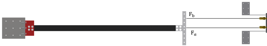
Figure 9: Elevated view of the test configuration and the pulling forces applied to the tip fixture.
