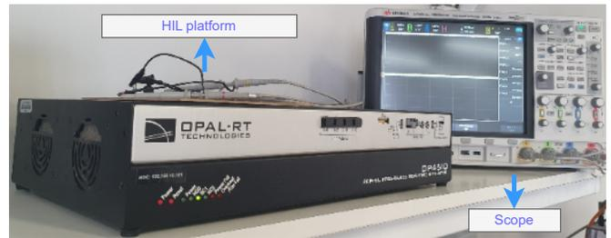
Fig. 11. OPAL-RT platform for HIL validation
