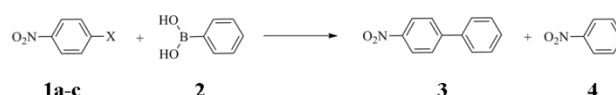
Scheme 1 The Suzuki-Miyaura and dehalogenation reactions ( 1a-c where X = Cl, Br and I respectively).
