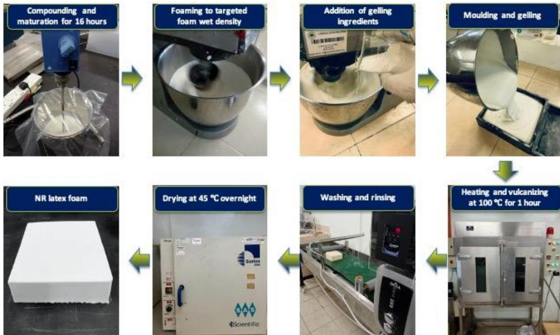
FIG. II. The different stages involved in the fabrication of NR latex foam using the Dunlop batch foaming process
