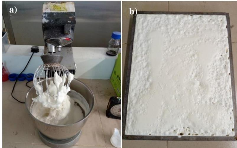
FIG. V. Failure during foaming process
