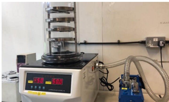
187 188 Figure 3. Image of freeze dryer and vacuum pump
