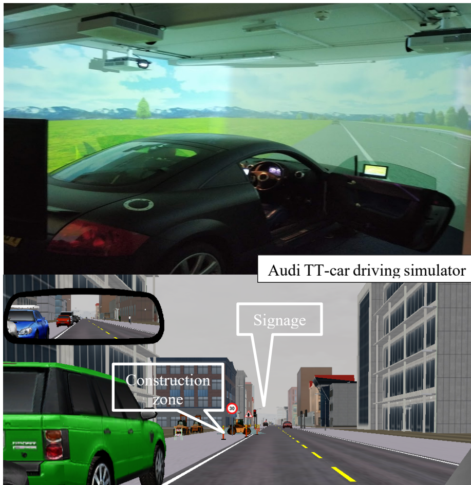
Figure A3 Experimental set up: fixed-base simulator and scenario at take-over request (design view in STISIM at 100ft after onset of TOR)
