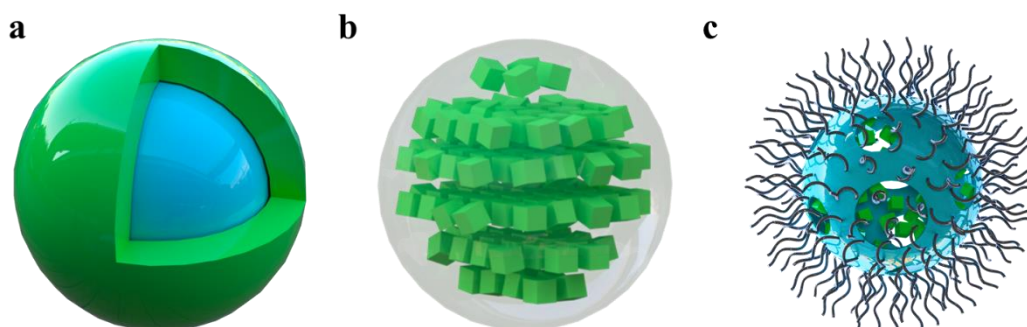
Figure 1 Schematic illustration of core/shell architectures, including a) CsPbBr 3 /Cs 4 PbBr 6 core/shell structure. Reproduced with permission. [37] Copyright 2018, RSC. b) CsPbBr 3 /SiO 2 modified by 2-methoxyethanol. Reproduced with permission. [38] Copyright 2017, Wiley-VCH. c) CsPbX 3 /MPMs/SiO 2 hybrid microspheres. Reproduced with permission. [39] Copyright 2019, Wiley-VCH.
