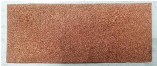
(b) Copper foam wick of vapour chamber
