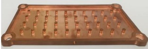
(a) Interior structure of vapour chamber without wick structure (Bottom plate)
