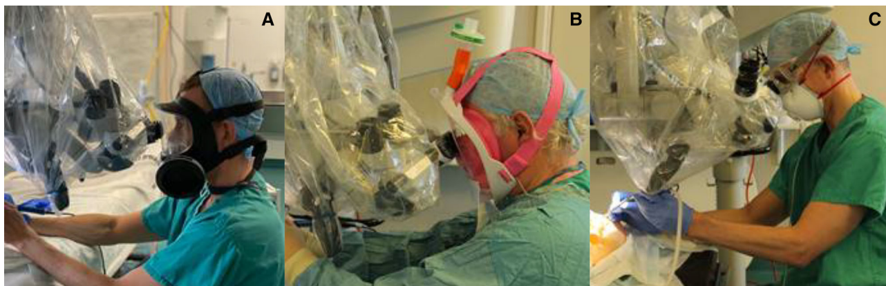
Fig. 1. PPE solutions subjected to an ergonomic evaluation. (A) Full-face respirator (Promask; 3M Scott, Monroe, NC). (B) Modified full-face snorkel mask that consists of a full-face mask, an appropriate medical-grade filter that captures viral particles, and a custom-made three-dimensional-printed adaptor that connects the two. 11 (C) FFP3 mask (3M 1863) and soft goggles (Bollé Coverall COVERSI) or spoggles (Bollé BAXTER RX) used as an ensemble. [Color figure can be viewed in the online issue, which is available at www.laryngoscope.com .]
