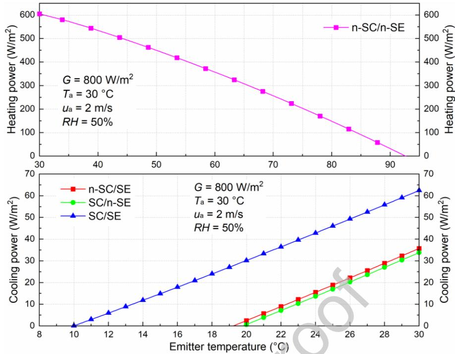
Fig. 5. Performance of the four RC modules in a daytime condition.
