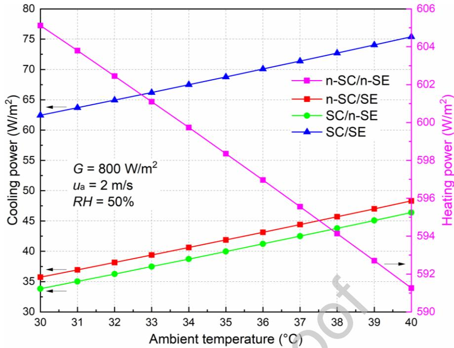
Fig. 7. Performance of the four RC modules at different ambient temperatures.
