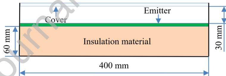
Fig. 2. Section structure of the radiative cooling module.
