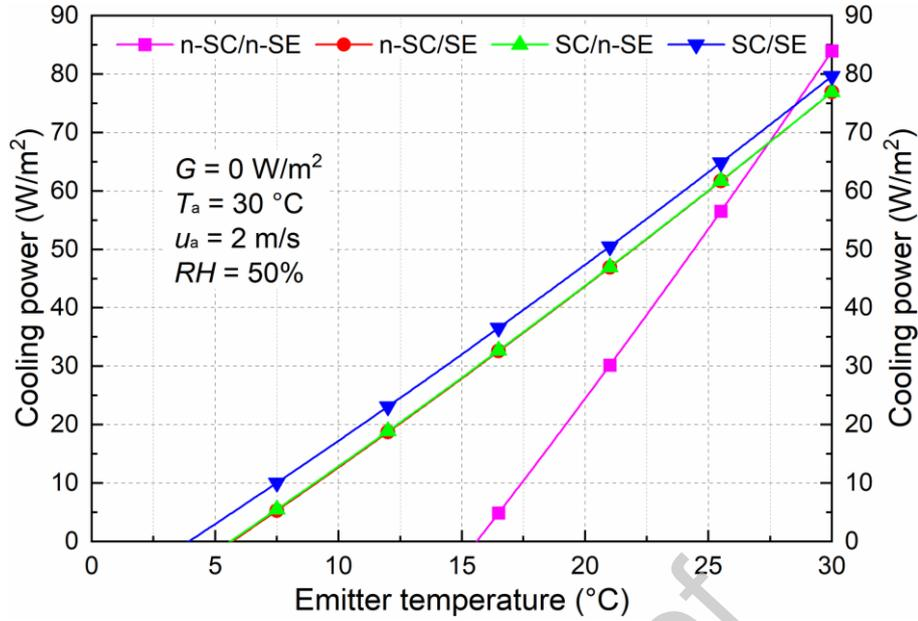
Fig. 6. Performance of the four RC modules in a nighttime condition.
