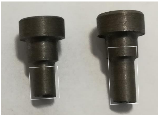
Fig. 5 Tested cast iron specimens under uniaxial tension
