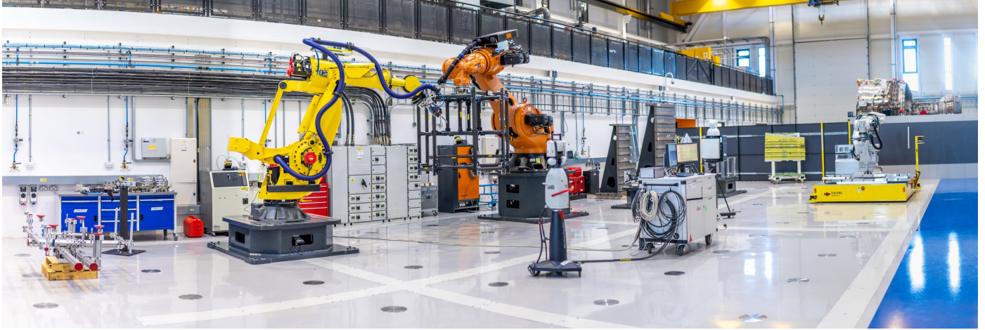
Figure 8: Omnifactory® - UK national training and research testbed for smart manufacturing system: Reconfigurable floor with calibrated floor points to locate robots within the facility
