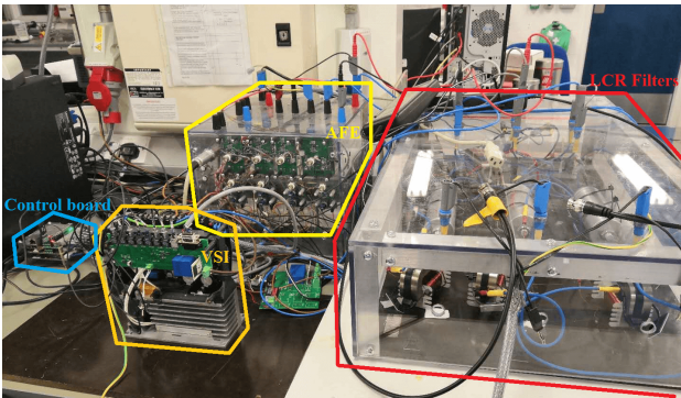
Fig. 5. Experimental rig of the VSI-AFE system
