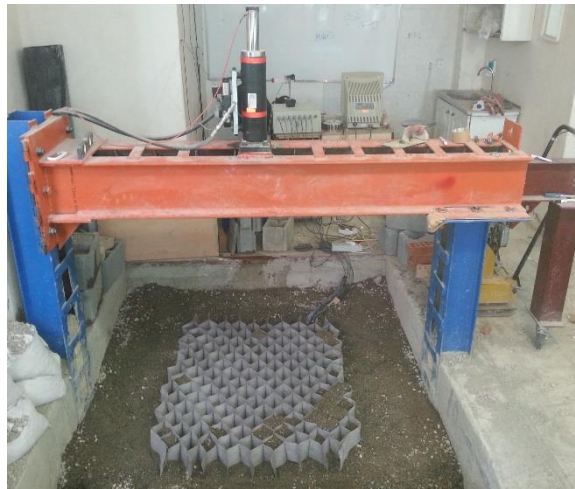
Fig. 3. A view of geocell (TDP Limited) spread over the pipe in the test pit
